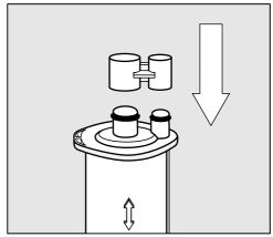
■ Seal the cartridge with the cap.
