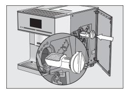
■ Fill the coffee scoop with ground coffee. Push the ground coffee drawer horizontally into the ground coffee chute.
