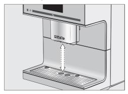
You can switch off spout adjustment. The central spout will then remain in the upper position while the drinks are being made. When a maintenance programme is being carried out the central spout will move to the height of the cleaning containers or into a maintenance position.
