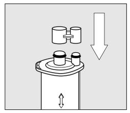
■ If you have switched on Automatic descaling, remove the descaling cartridge. Put the cap on the descaling cartridge.
