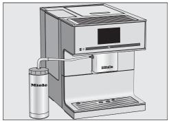
■ Place the milk flask beside the coffee machine. Connect the other end of the milk tube to the central spout.
